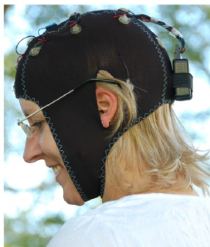
Fig. 1. The mobile EEG system as proposed by Debener et al. (2012) consists of an amplifier-power supply unit, which is attached to the cap at the back of the head (weight 48 g, size 40 × 40 × 21 mm).
