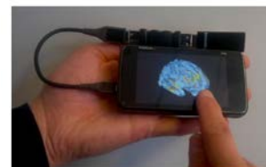
Fig. 3. A user interacting with a 3D model of the brain using the handheld brain scanner device with touch-based interaction.
