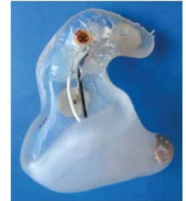
(b) An earplug with electrodes and connector (opposite view of Figure 1(a)). Electrode ERE is visible.
