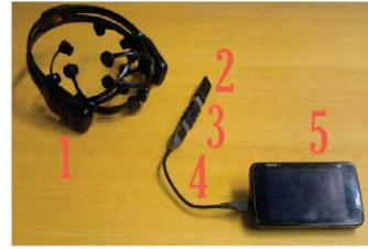
Fig. 1. Handheld brain scanner components. Emotiv EPOC wireless EEG headset (1), Emotiv Receiver module with USB connector (2), USB connector and adapter (3+4), and Nokia N900 mobile phone. The total cost of the system is less than USD1000.
