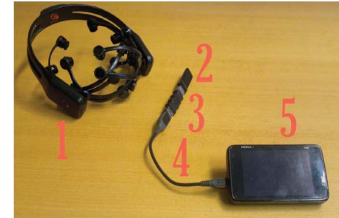
Fig. 1. Handheld brain scanner components. Emotiv EPOC wireless EEG headset (1), Emotiv Receiver module with USB connector (2), USB connector and adapter (3+4), and Nokia N900 mobile phone. The total cost of the system is less than USD1000.
